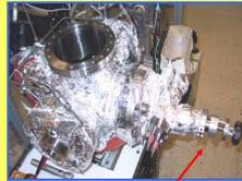
Manipulator (for moving the substrate)
