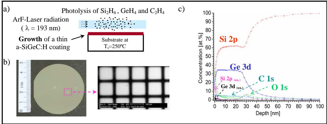
Fig.1 (a) Scheme of the LCVD process, (b) views of uniform coatings deposited on a 2'' Si wafer and on selected regions ( $200 \times 200 \mu\text{m}^2$  squares), (c) XPS depth profile analysis of an SiGeC films on a thin  $\text{SiO}_2$  film
