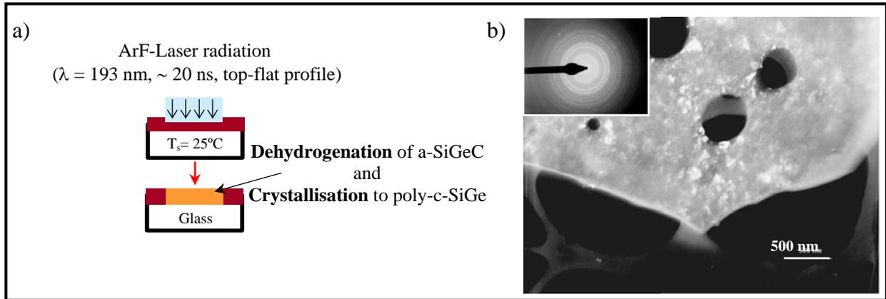
Fig.2 (a) Scheme of the dehydrogenation and the ELC process, (b) TEM electron diffraction and plane view dark field image showing fine grained material (coherence length determined by XRD is 10 – 20 nm).
