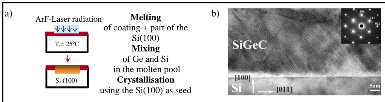
Fig.3 (a) Scheme of the PLIE process, (b) High resolution cross section TEM image of a heteroepitaxial SiGeC film on Si (100), with corresponding electron diffraction pattern.
